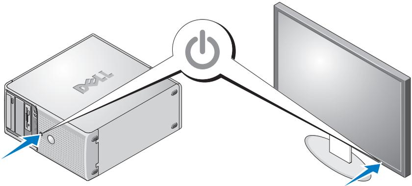
Press the power button on the system and the monitor. The power indicators should light. Adjust the monitor's controls until the displayed image is satisfactory.
