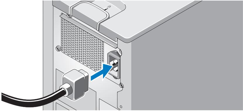
Connect the system's power cable to the system. Next, plug the other end of the power cable into a grounded electrical outlet or a separate power source such as an uninterruptible power supply (UPS) or a power distribution unit (PDU).
